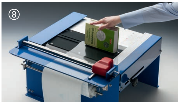
Place the book in a central position on the squeegee and leave a top and bottom overlap of film of 2 cm.
