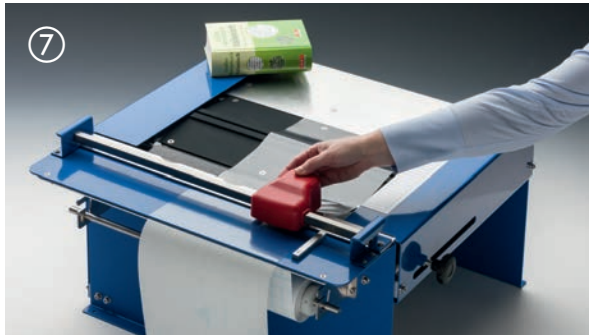
Now take hold of the cutter head to cut the film.
