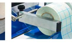
Secure the roll with the tape holder and tighten the screw. The tape can be cut off with a light diagonal, downward motion onto the cutting blade.
